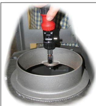
Fig. 4 Remove the bolts holding the top flue outlet.
