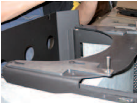
26. The pins should face forward so they fit the holes in the top soapstone element. The slotted holes allow for adjustment.
