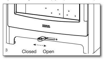
fitted to ensure that the air control slider cannot be closed beyond 33% for Ambition 5 and 42% for Ambition 8 of its fully open position. A permanent amount of air will therefore enter the firebox to feed the fire producing negligible amounts of smoke and unburnt hydrocarbons. The appliances will only be considered as an exempt appliance if this stop is in place.
