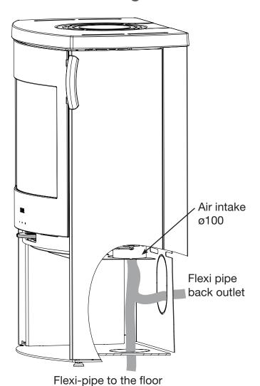
When installing external air supply, connect the air intake to the direct air pipe using flexi-pipe, both from the floor or behind the stove.
