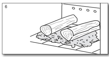
Now open the combustion air completely. If the stove and/or chimney cools down too much, it may be necessary to have the door ajar. The wood will then ignite within a very short time (Typically 1 to 3 minutes). Once the fuel is Ignited. Close the door and regulate the air back to operating air. When the fire is well established, you can now regulate the operating air to the desired combustion level.
