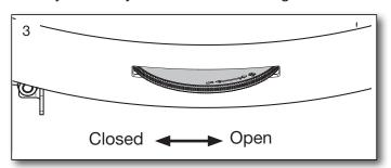
exempt for use in smoke control areas throughout the UK when burning dry wood logs. To comply, a permanent stop is fitted to ensure that the air control slider cannot be closed beyond 35% of its fully open position. A permanent amount of air will therefore enter the firebox to feed the fire producing negligible amounts of smoke and unburnt hydrocarbons. The appliances will only be considered as an exempt appliance if this stop is in place.
