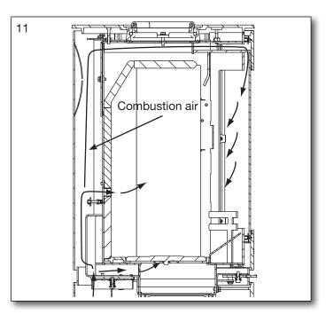
Nominal fluegas temperture: 257° relative to 20°C. Flue gas flow is: 3.9 g/sec. Corresponding to 14.8 m³/hr of combustion air by burning 1.06 kg of wood.
