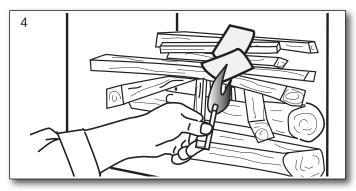
Fully open the combustion air and leave the door ajar (about 1 cm open).
