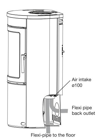
When installing external air supply, connect the air intake to the direct air pipe using flexi-pipe, both from the floor or behind the stove.
